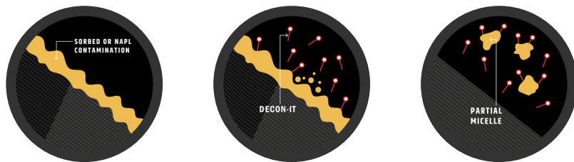
The above images show the DECON-IT® mechanism selectively removing surface sorbed contaminants with consistent results.
